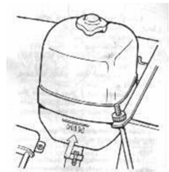
Fig 38 Cooling system expansion tank
